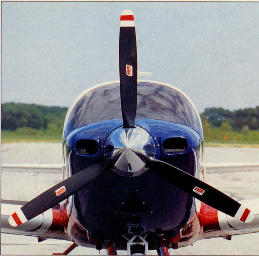
The Ovation cowl is noteworthy for its tiny cooling inlets. Cowl flaps are unnecessary, according to Mooney. Negative pressure helps scavenge exhaust gases from small-diameter, faired pipes.
