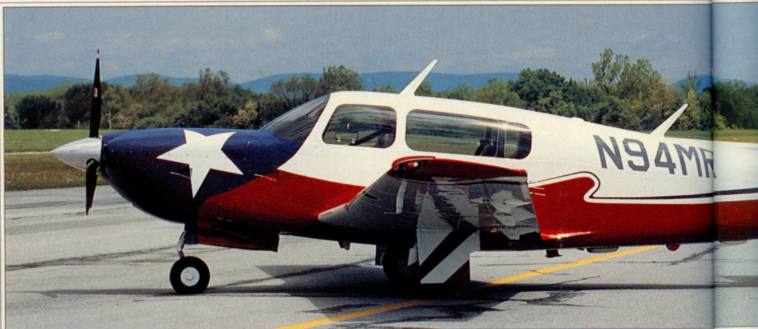
The new tapered cowl (above) is lower and shaplier than that of other Mooneys. The panel is light gray with silkscreened placards. Switches for exterior lights (above, right) have been moved off the panel to an overhead console. Rear seats (below, right) recline and fold down.
