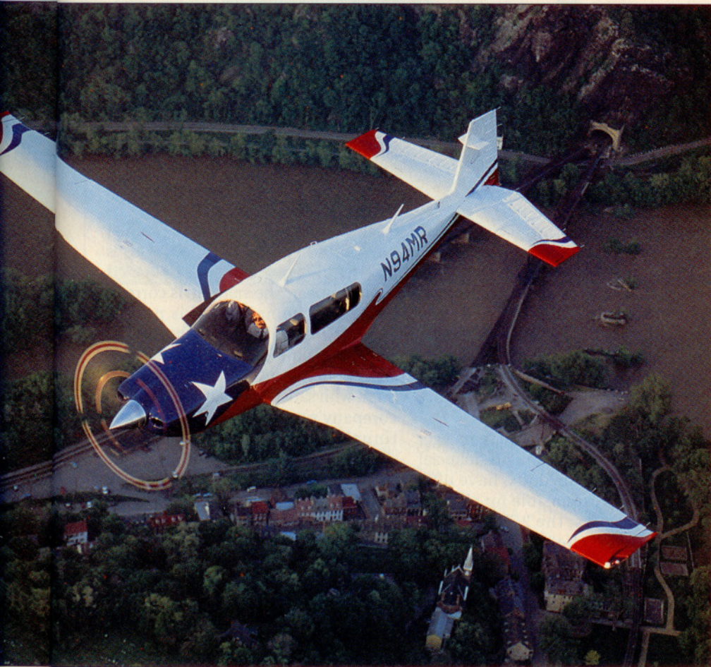
The Ovation cowl is noteworthy for its tiny cooling inlets. Cowl flaps are unnecessary, according to Mooney. Negative pressure helps scavenge exhaust gases from small-diameter, faired pipes.
